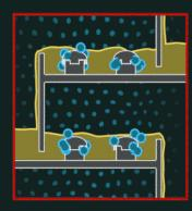
The distilled products are then piped off from the different levels of the tower. These separated products are called **fractions** or **distillates.**
